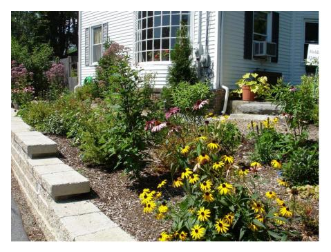
Completed Rain Garden @ Broad Meadow Brook Wildlife Sanctuary, Worcester, MA. A good soil mix for rain gardens is 50-60% sand, 20-30% topsoil & 20-30% compost. Shredded hardwood as mulch keeps the soil moist and ready to soak up rain and reduces maintenance needs.
