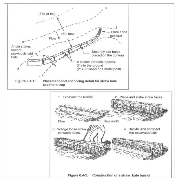
Installation of hay-bales for sediment retention purposes
