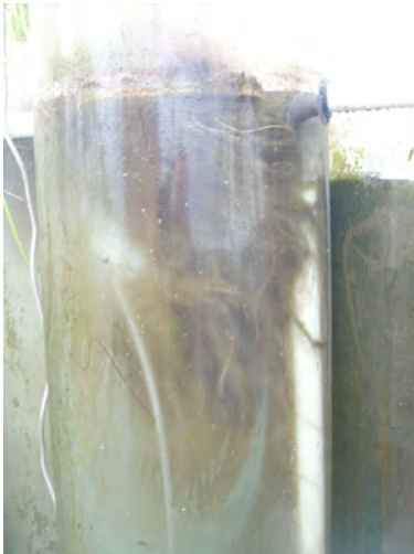
Figure 1 Clear tank walls maximize solar penetration within the aquatic cells.
