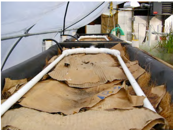
Figure 4 Mycofilter troughs create a “trickle-filter” pathway for exposing contaminants to mycelium.
